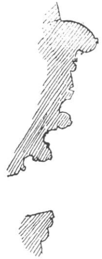
Fig. 234 Profiles from (above) main doorway (below) cornice of belfry.
