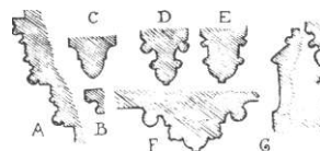
Fig. 121 Profiles: A. west doorway; B. abacuses of its capitals; C. ribs of the porch; D. ribs of the refectory; E. transverse ribs of the refectory; F, G. columns of the refectory; H. abacuses of the undercroft; I. ribs of the cloisters.
