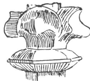
Fig. 169 Finial on the buttresses.
